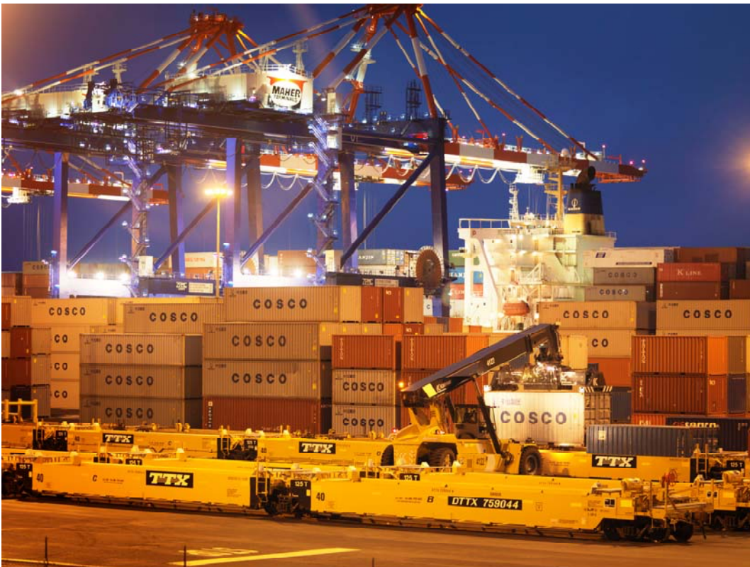
Kalmar reach stackers loading containers onto railcars during nightshift. The maximum dwell time of offloaded containers is 48 hours.
